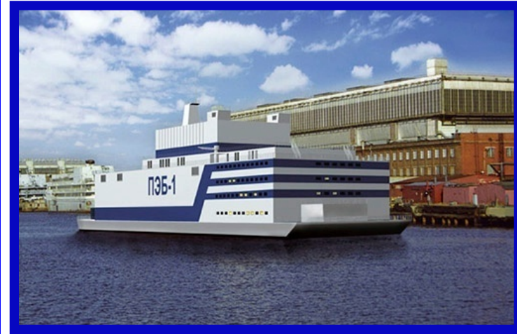
Floating power-generating unit with a KLT-40S reactor system for electricity and water desalination
